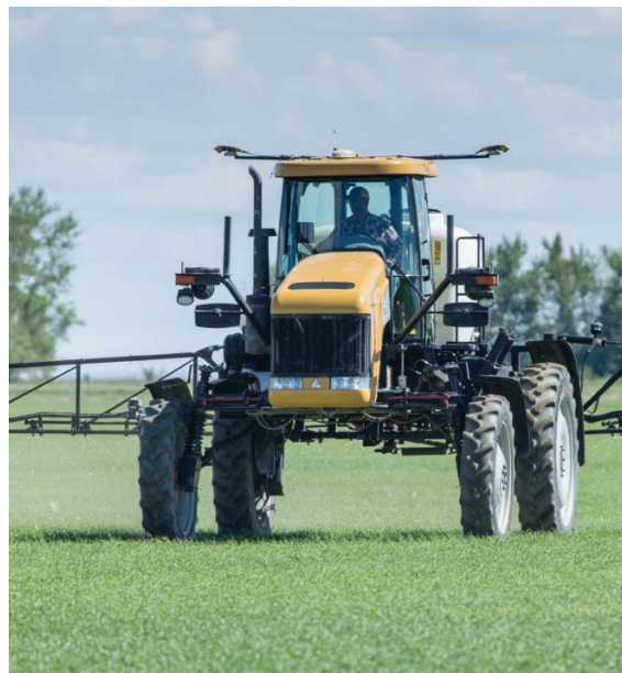
Pic.2 A sprayer with a spray control system for precise application of agents. Source: https://www.topconpositioning.com/content/dam/topcon_digital_asset_hub/collateral/brochures/Crop_Spec_Broch_7010-0957_TEAM_EN_US_HiRes.pdf
