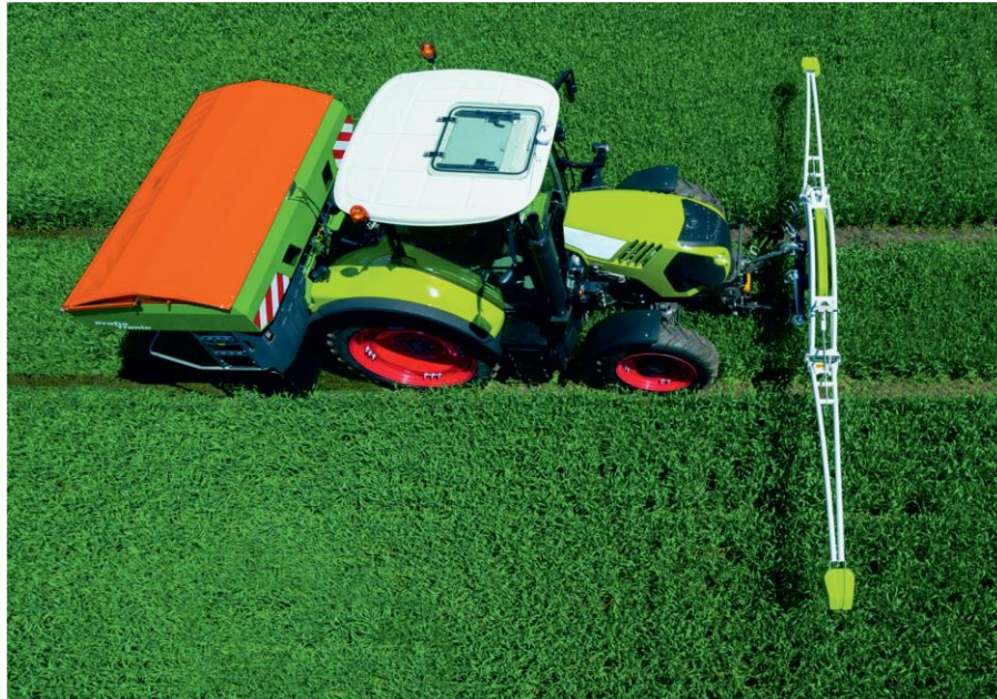
Photo. 1 Optical sensors for precision fertilization placed in the heads on the right and left side arm mounted on the front suspension of the tractor. Source: Precision Fertilization Poznań 2018
